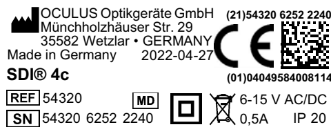
Fig. 2-1: Rating plate SDI® 4c
